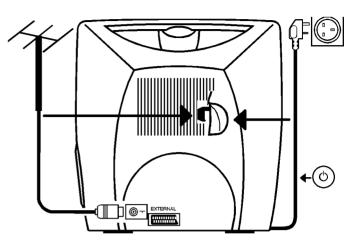
1 Insert the aerial plug into the received socket.
